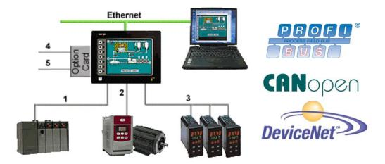
With three serial ports standard, (up to five with optional expansion card), and an Ethernet port capable of running four protocols, the G3 is the most powerful communications platform available today. Pick the best-in-class PLC, drive, temperature controllers, etc. for your next machine. The Red Lion G3 will make sure they communicate seamlessly to one another.
