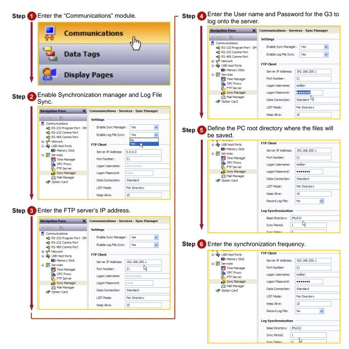
The G3 will synchronize the content of the CompactFlash card with the FTP server as defined in the Sync period.
