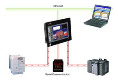
With the G3's powerful protocol converter, you have the ability to exchange data between any and all connected devices. With a few clicks of the mouse, you can map a setpoint from a PLC to a variable speed drive, or provide a PLC program with information as to the status of a PID controller.
