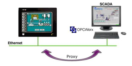
Red Lion's OPCWorx is a configuration tool for our OPC servers. This easy-to-use software allows you to create and configure an OPC server to communicate with the G3 series HMI, the Data Station Plus or the Enhanced Master, as well as devices that support Modbus. Any SCADA package that provides OPC connectivity can then access the G3's tags via their given name.
