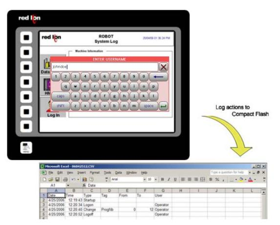
The Security manager provides multi-user, multilevel password protection. The advanced security logger tracks operator actions as well as any data changes for later review.
