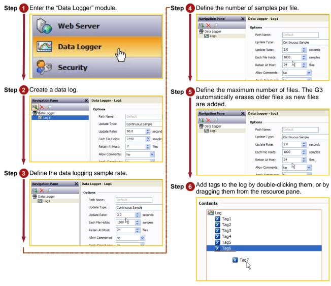
In this example, the G3 will log the last 24 hours of data, with each file representing one hour of samples.
