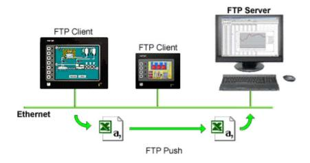
Synchronize log and event files from the HMI to a PC for permanent storage and further analysis. The G3's FTP synchronization can be performed automatically or on demand.
