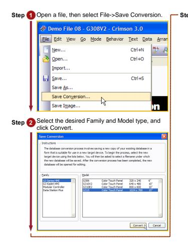
• Step 3 Provide a new name for the converted file.
