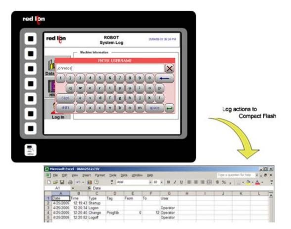
The Security Manager provides multi-user, multilevel password protection. The advanced security logger tracks operator actions as well as any data changes for later review.
