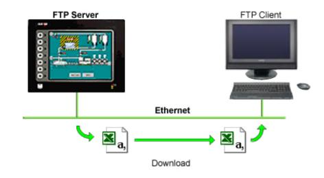
Connect to the HMI via FTP to download or upload any files available on the CompactFlash Card. Easily update recipe files or access log information from your web browser, Windows Explorer or any FTP client software.
