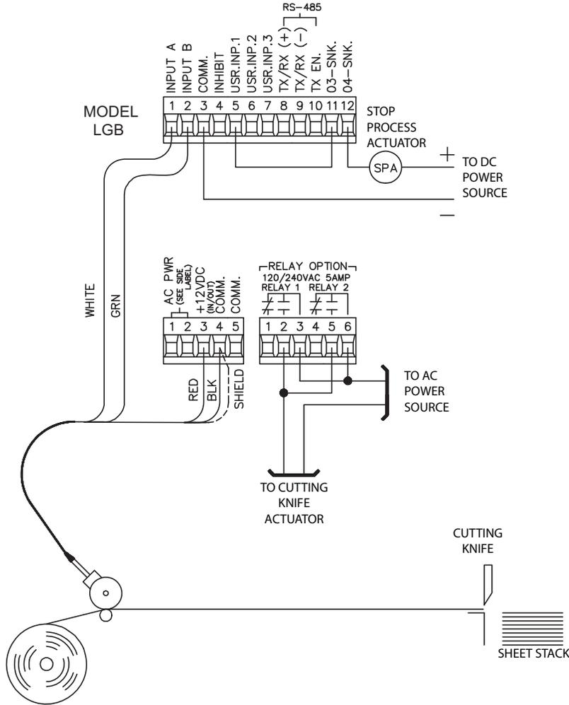
Preset value  $P_1$  (*Process count*) is programmed for the first length to be cut for the order and Preset value  $P_2$  (*Process count*) for the second length.
